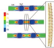
ordering, the researchers found that it cannot alone explain the structural periodicity. Additional calculations show that epitaxial attachment of Ag<sub>2</sub>S and CdS in the nanorod leads to significant amounts of strain due to a substantial lattice mismatch, re-
